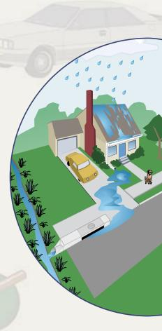
s stormwater flows over driveways, lawns, and sidewalks, it picks up debris, chemicals, dirt, and other pollutants. Stormwater can flow into a storm sewer system or directly to a lake, stream, river, wetland, or coastal water. Anything that enters a storm sewer system is discharged untreated into the waterbodies we use for swimming, fishing, and providing drinking water. Polluted runoff is the nation's greatest threat to clean water.
